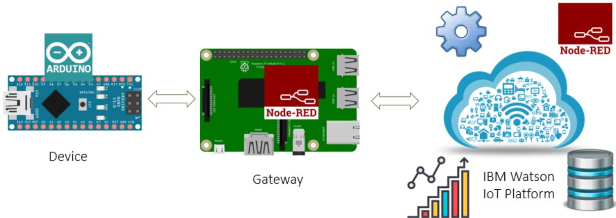
Figure 2 Basic Architecture of Smart Farming using IoT
